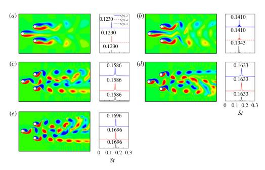
FIGURE 23. Vorticity fields (left) and spectra of the lift coefficients (right) at L/D = 5.0. (a-e) Represent the results at Re = 50, 75, 125, 150 and 175, respectively.
