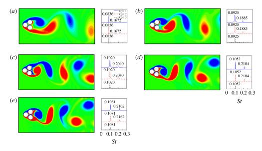
FIGURE 14. Vorticity fields (left) and spectra of the lift coefficients (right) at L/D = 1.2. (a-e) Represent the results at Re = 50, 75, 125, 150 and 175, respectively.
