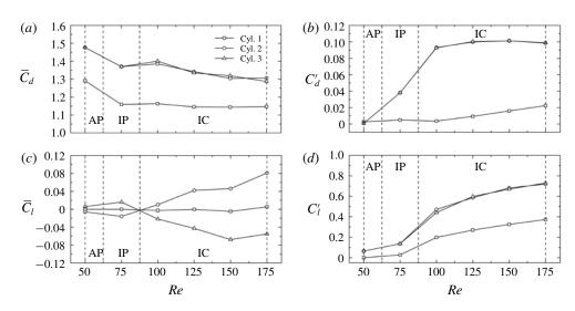
FIGURE 22. Fluid forces acting on three cylinders at L/D = 5.0.
