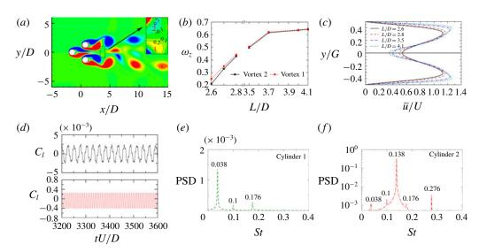
FIGURE 6. Flow and force characteristics in the anti-phase regime. (a) Vorticity contours at L/D = 2.6. Vortices 1 and 2 marked in (a) are shed from the upstream cylinder. (b) The maximum z-vorticity (absolute value) of the vortex pair shed from the upstream cylinder. (c) The time-averaged gap flow streamwise velocity profiles at L/D = 2.6-4.1. (d) Times histories of the lift coefficients at L/D = 2.7. (e) Lift spectrum of Cylinder 1. (f) Lift spectrum of Cylinder 2.
