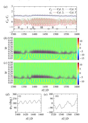
FIGURE 19. Flow past three cylinders at Re = 175 and L/D = 2.5. (a) Time histories of the drag and lift coefficients of two downstream cylinders, (b) the real part of the wavelet transform of the lift coefficient of Cylinder 2, (c) the real part of the wavelet transform of the lift coefficient of Cylinder 3 and (d) the phase difference between the two downstream cylinders. Regions I, II, III denote regimes of the flip-flopping flow, transition and anti-phase flow, respectively.
