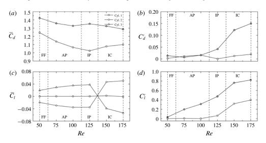
FIGURE 20. Fluid forces acting on three cylinders at L/D = 4.0.
