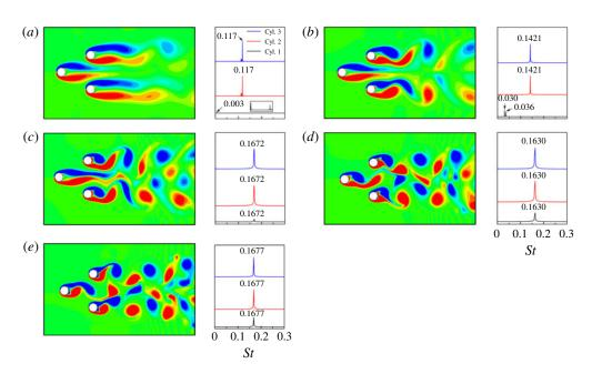
FIGURE 21. Vorticity fields (left) and spectra of the lift coefficients (right) at L/D = 4.0. (a-e) Represent the results at Re = 50, 75, 125, 150 and 175, respectively.
