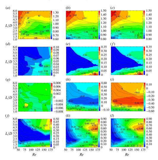
FIGURE 25. Fluid forces acting on three cylinders versus Re (= 50-175) and L/D (= 1.0-6.0). The rows, from left to right, represent the results of Cylinders 1, 2 and 3, respectively. (a-c) Mean drag, (d-f) r.m.s. drag, (g-i) mean lift and (j-l) r.m.s. lift.
