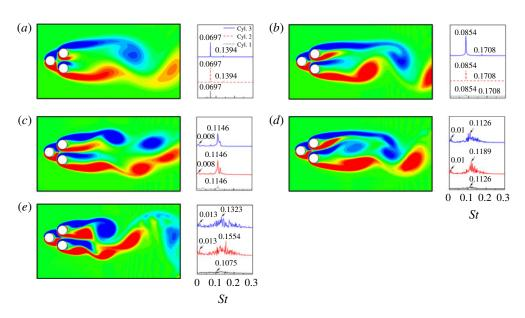
FIGURE 16. Vorticity fields (left) and spectra of the lift coefficients (right) at L/D = 1.6. (a-e) Represent the results at Re = 50, 100, 125, 150 and 175, respectively.
