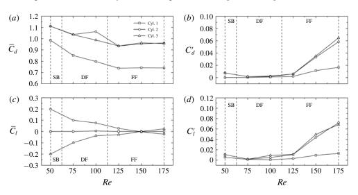
FIGURE 15. Fluid forces acting on three cylinders at L/D = 1.6.
