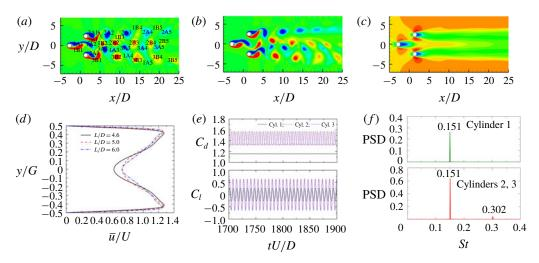
FIGURE 8. Instantaneous vorticity fields at L/D = 4.8 (a) and 5.0 (b). (c) Time-averaged streamwise velocity field at L/D = 4.8. (d) Time-averaged streamwise velocity profiles in the gap of two downstream cylinders. (e) Time histories of the drag and lift coefficients and (f) lift spectra of three cylinders at L/D = 4.8. The arrow in (a) indicates the upward flow generated between 2A2 and 2B1.
