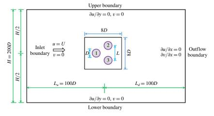
FIGURE 1. The computational domain and boundary conditions for the flow past three cylinders in an equilateral-triangular arrangement.
