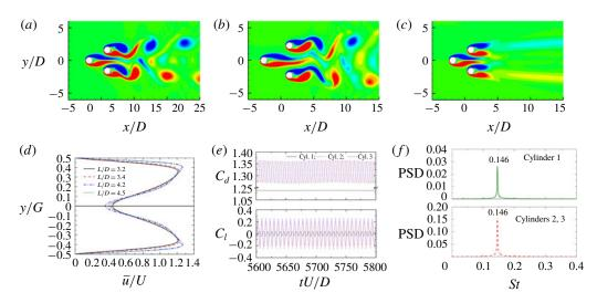
FIGURE 7. Instantaneous vorticity fields at L/D = 3.2 (a) and 4.5 (b). (c) Time-averaged vorticity field at L/D = 3.2. (d) Time-averaged streamwise velocity profiles in the gap of two downstream cylinders. (e) Time histories of the drag and lift coefficients at L/D = 4.5. (f) Lift spectra of three cylinders at L/D = 4.5.
