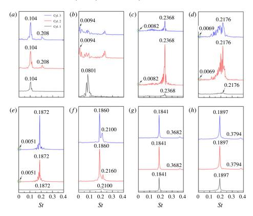
FIGURE 29. Spectral analyses of the lift coefficients of three cylinders at Re = 300 and (a) L/D = 1.2, (b) L/D = 1.6, (c) L/D = 2.0, (d) L/D = 2.5, (e) L/D = 3.0, (f) L/D = 3.5, (g) L/D = 4.0 and (h) L/D = 5.0.
