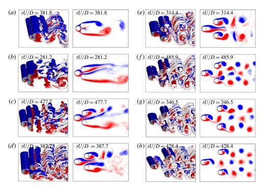
FIGURE 27. The vorticity contours of flow past three cylinders at Re = 300 and (a) L/D = 1.2, (b) L/D = 1.6, (c) L/D = 2.0, (d) L/D = 2.5, (e) L/D = 3.0, (f) L/D = 3.5, (g) L/D = 4.0 and (h) L/D = 5.0. Isosurfaces  $\lambda_2 = -0.2$ . The second and fourth columns represent the spanwise-averaged vorticity contours.
