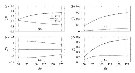
FIGURE 13. Fluid forces acting on three cylinders at L/D = 1.2.
