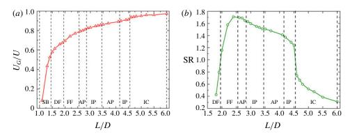
FIGURE 12. (a) The normalized time- and space-averaged streamwise velocity  $(U_G/U)$  of the gap flow. (b) The normalized maximum shearing rate (SR = (D/U)(du/dy)) of the gap flow profile between two side peaks. The flow patterns are separated by the dashed line.
