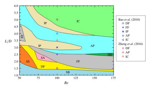
FIGURE 24. Flow regimes of flow past three circular cylinders in the parametric space of Re (= 50-175) and L/D (= 1.0-6.0). The boundary between two adjacent flow patterns is approximately determined by using the midpoint of two adjacent data points. SS, steady symmetric flow; SA, steady asymmetric flow; HB, hybrid flow.
