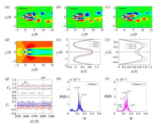
FIGURE 4. Flow and force characteristics at L/D = 2.2. (a-c) Correspond to the upward deflected, parallel and downward deflected gap flow. (d) The time-averaged streamwise velocity. (e) The time-averaged streamwise velocity profiles at 1D behind the centres of two downstream cylinders. (f) The time-averaged streamwise velocity profiles in the gap of two downstream cylinders. (g) Time histories of the drag and lift coefficients. (h) Spectra of the lift coefficients.
