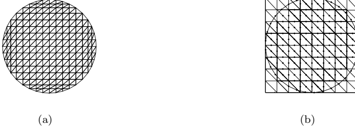
Figure 4: (a) A finite element triangulation of \overline{B_{jh}(t)} . (b) Set of nodes inside \overline{B_{jh}(t)} from the velocity grid and control points on \partial B_j(t) to enforce rigid body motion by the collocation method .
