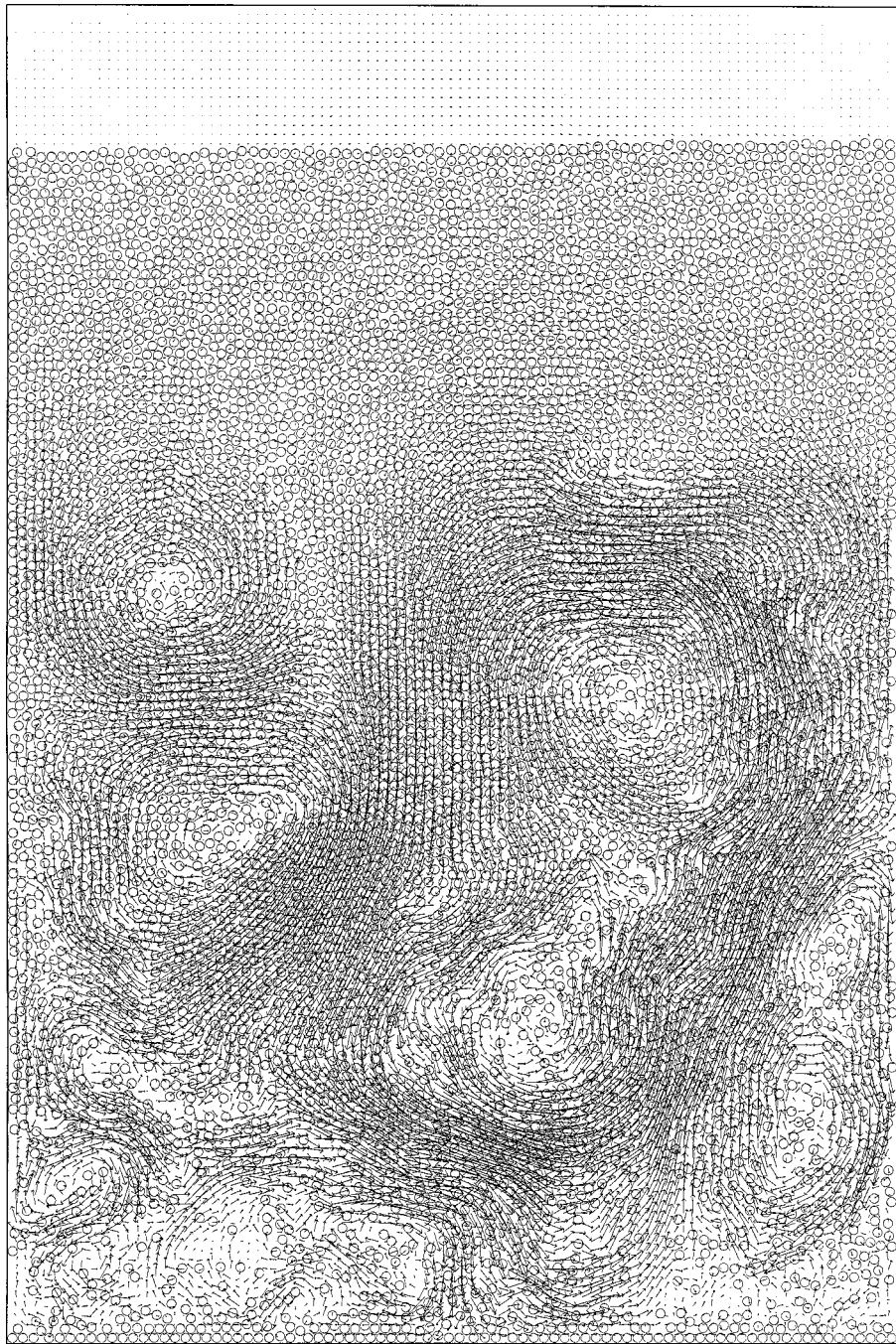
FIG. 8.34. Sedimentation of 6400 particles: t = 3 .
