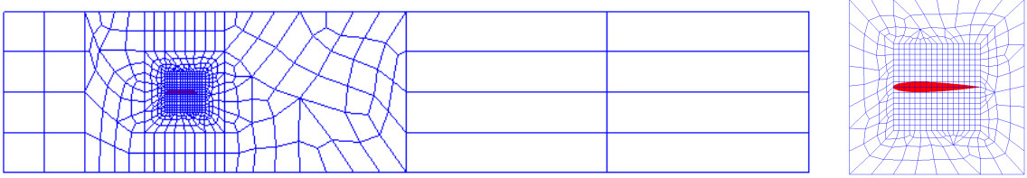
Figure 10: Coarse mesh for flow around a NACA0012 airfoil (left is the global mesh, right is a local zoom covering the airfoil at LEVEL = 1)
